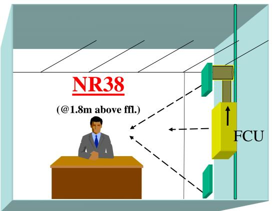
FCU @ 210 l/s & 30 Pa With room absorption, ductwork, plenum & grille.
