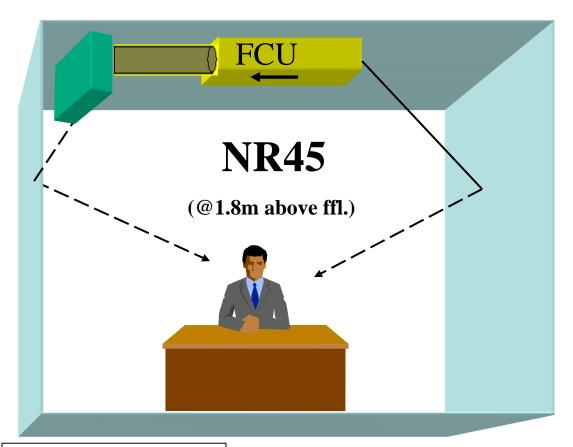
FCU @ 240 l/s & 30 Pa With Room absorption 1 m of Acoustic Ductwork, Plenum & Grille No Ceiling
