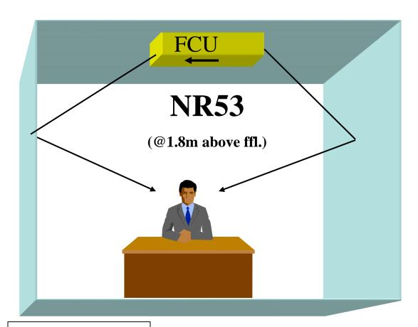
FCU @ 240 l/s & 30 Pa No Room absorption No Ductwork No Ceiling
