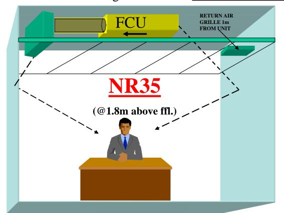
FCU @ 240 l/s & 30 Pa With room absorption 1 m of acoustic ductwork, plenum & grille. With 10mm insulated pan tile ceiling.
