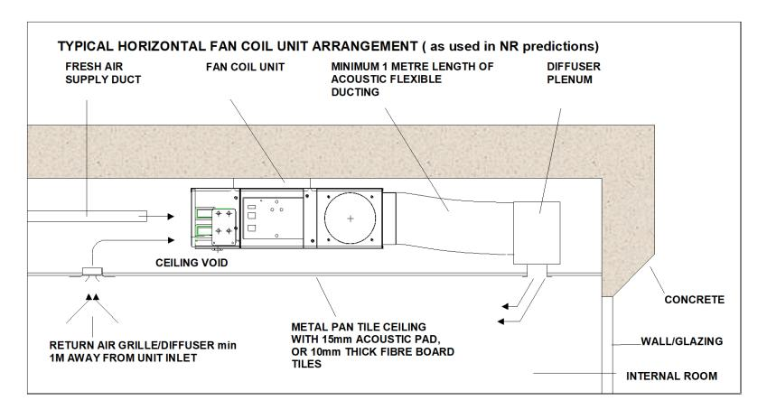
To ensure that the installed noise levels achieve the suppliers quotations, many manufacturers include an installation specification like this, to ensure that the units are not installed into non-standard applications. Follow best practice and the final system will achieve the specified noise performance.
