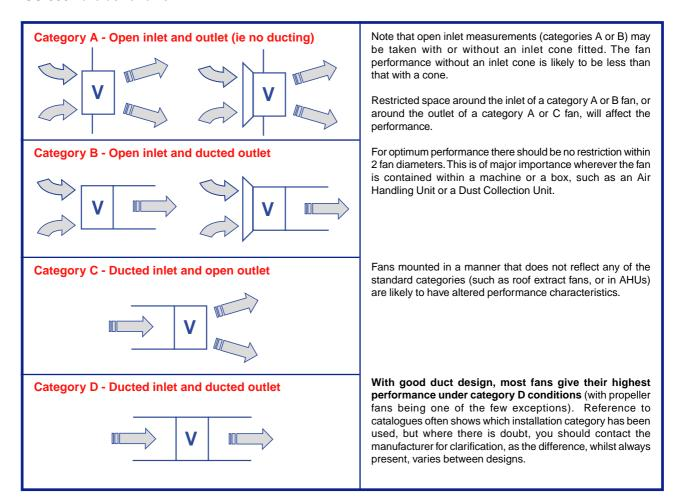
Ducting modifies the air flow into and out of the fan, so the design of ducting connected to the fan inlet and/or outlet is extremely important.
